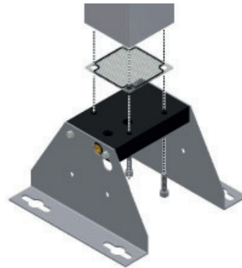
Removing base plate
