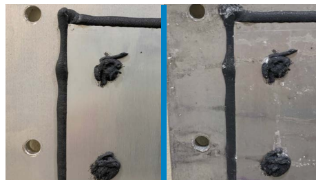
CHO-BOND 1018 before (left) and after (right) 1,000 hours salt fog exposure.
