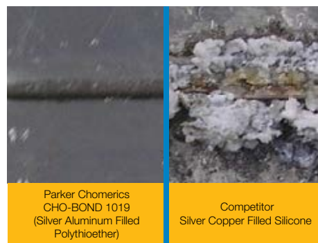
After 1,000 hours exposure in a ASTM B117 salt fog environment, CHO-BOND 1019 panel (left) shows no change where competitive product shows corrosion (right).
